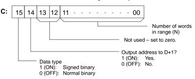
If bit 14 of C is ON, values above #8000 are treated as negative numbers, so the results will differ depending on the specified data type. Be sure that the correct data type is specified.
